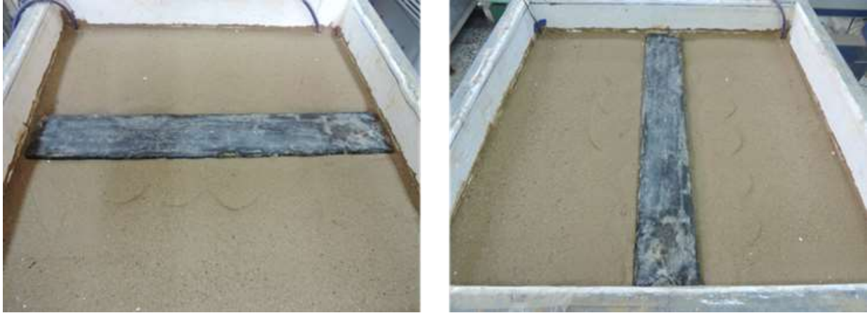
Figure 9: Geocell reinforcement within model test.
